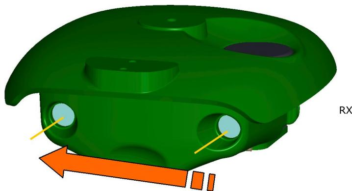
Figure 4 – Standing behind receiver: Positive velocity for cars travelling left to right
