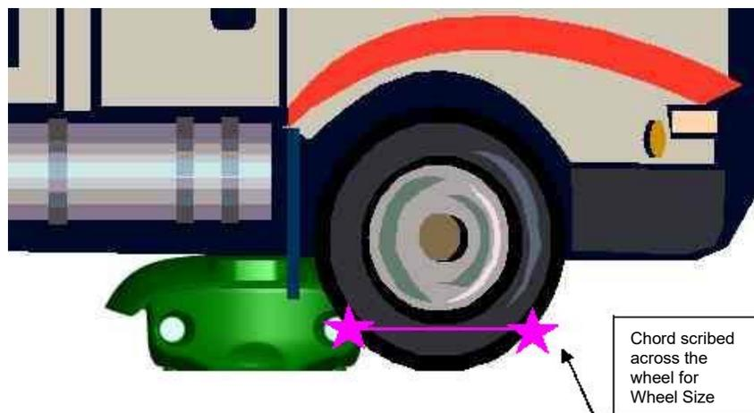
Figure 7 – Wheel Size Measurement
